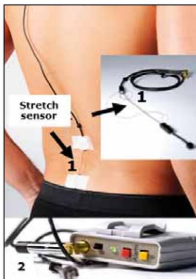
Fig. 13. The BodyGuard, 1 the stretch sensor, 2. the measurement, alarm and storage unit.
